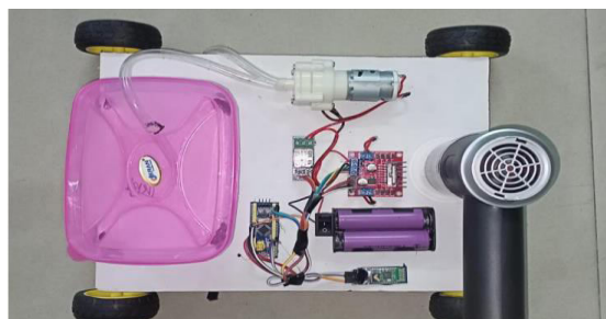
Figure.2. Experimental setup of the proposed Bluetooth Controlled Automatic Street Cleaning Robot
